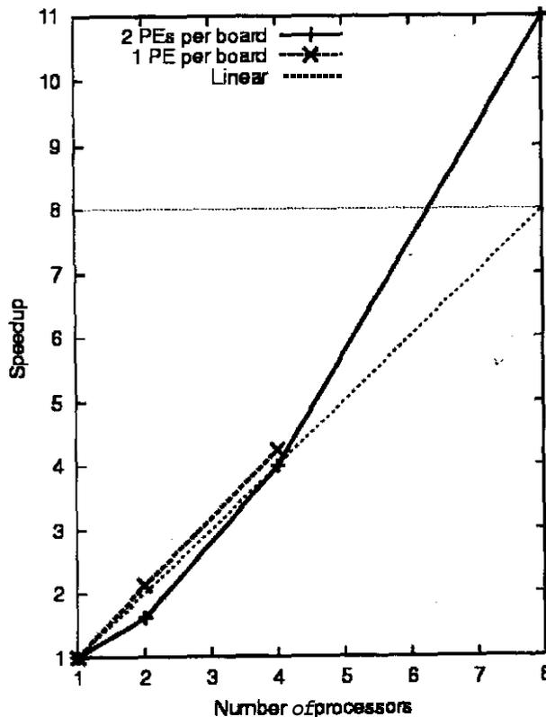
Figure 4. Speed-up of multigrid code on Flosolver.
