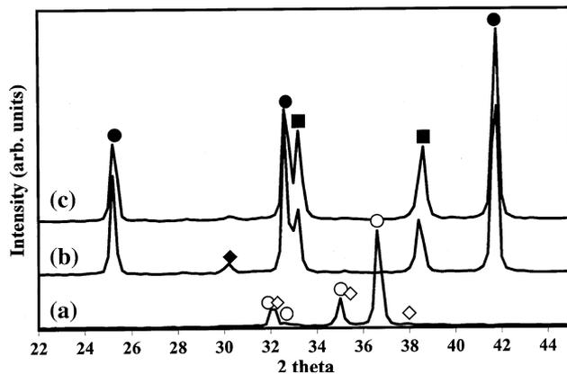
Fig. 2—XRD patterns of the stoichiometric  $ZrB_2$ - $ZrC$  composites at 40 MPa, 1200 °C for 30 min: (a) starting powder mixture, (b) composite with 1 wt pct Ni, and (c) composite without Ni (●— $ZrB_2$ , ■— $ZrC$ , ○—Zr, ◇— $B_4C$ , and ◆— $ZrO_2$ ). Note that owing to the coverage of  $B_4C$  particles by the heavy element zirconium, during mixing, the peaks for  $B_4C$  are not visible.
