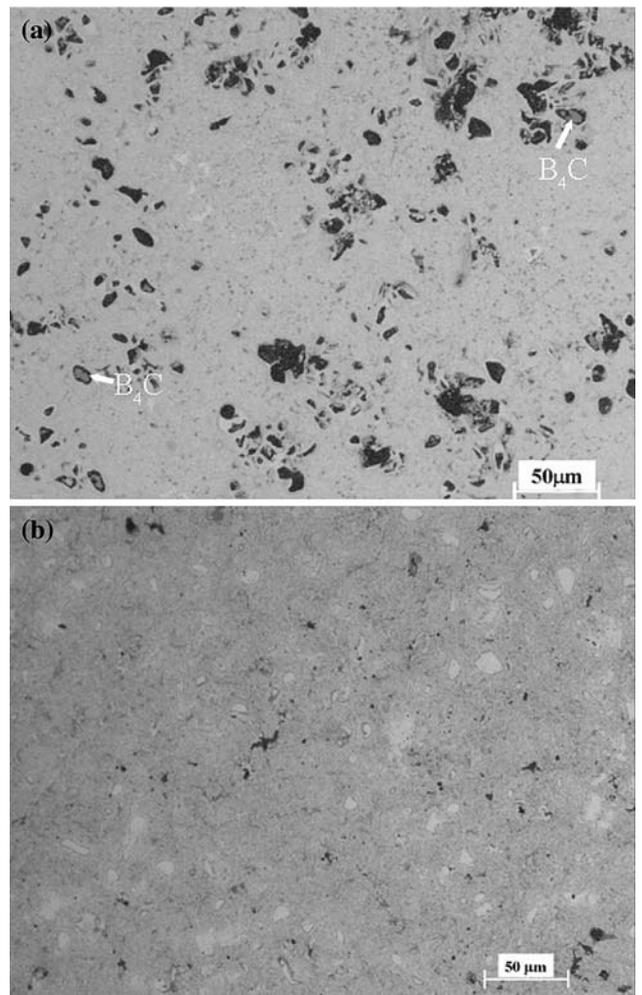
Fig. 8—Optical micrographs of the  $ZrB_2-ZrC_{x-0.67}$  composites produced at 40 MPa, 1200 °C for 30 min: (a) without Ni showing unreacted  $B_4C$  particles and (b) with 1 wt pct Ni showing completion of reaction. The dark regions are pores.
