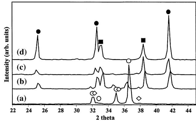
Fig. 6—XRD patterns of the nonstoichiometric  $ZrB_2$ - $ZrC_x$  composites produced with 1 wt pct Ni: (a) unreacted powder mixture, (b) —/1000 °C/5 min, (c) 40 MPa/1000 °C/30 min, and (d) 40 MPa/1200 °C/30 min (●— $ZrB_2$ , ■— $ZrC_x$ , ○—Zr, and ◇— $B_4C$ ).
