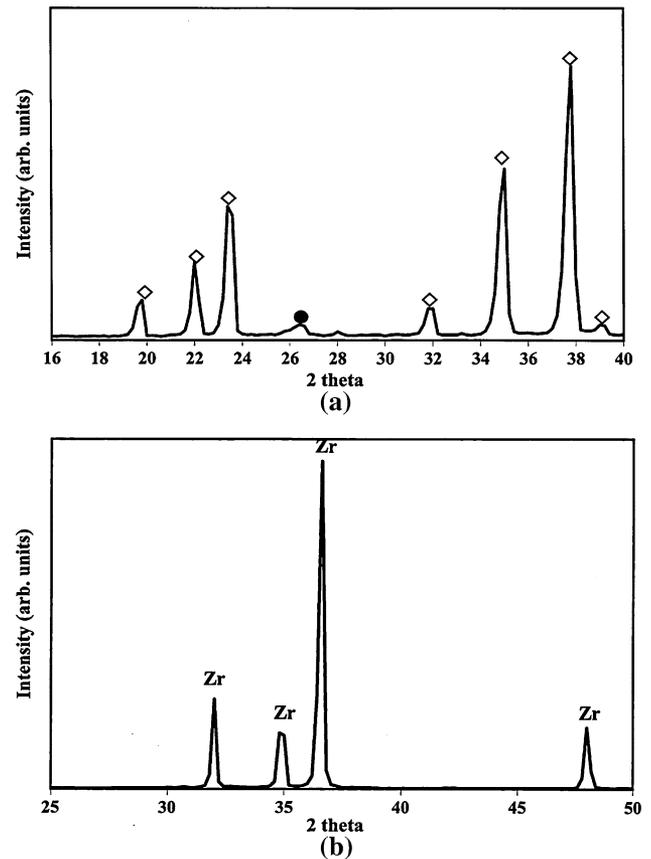
Fig. 1—XRD patterns of the starting powders: (a)  $\text{B}_4\text{C}$  ( $\diamond$ — $\text{B}_4\text{C}$  and  $\bullet$ —graphite) and (b) Zr. The starting  $\text{B}_4\text{C}$  powder shows a small graphite impurity peak.
