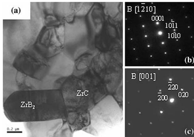
Fig. 7—(a) Bright-field TEM micrographs of  $ZrB_2-ZrC_{x-0.67}$  composite produced at 40 MPa, 1400 °C for 30 min (1 wt pct Ni) with selected area electron diffraction patterns for the (b)  $ZrB_2$  and (c)  $ZrC$ .
