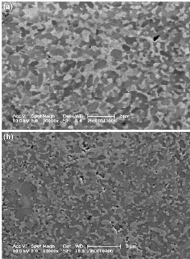
Fig. 10—SEM micrographs of the etched nonstoichiometric  $\text{ZrB}_2\text{-ZrC}_{x-0.67}$  composites produced at 40 MPa, 30 min with 1 wt pct Ni: (a) 1200 °C and (b) 1400 °C. The dark grains are  $\text{ZrB}_2$  and the light ones are  $\text{ZrC}_{x-0.67}$ . Both phases display grain sizes in the sub-micron range.
