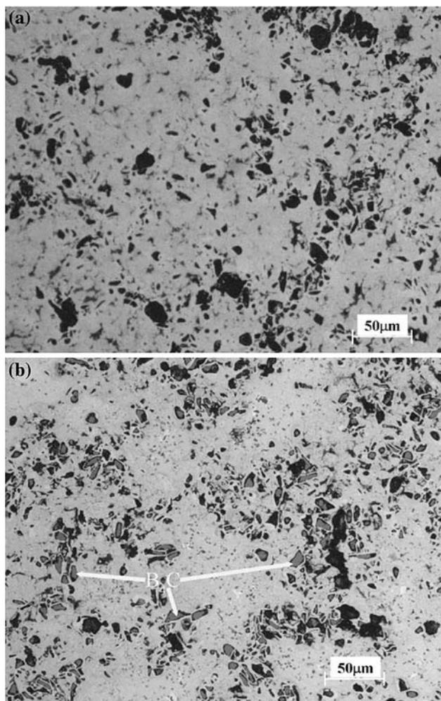
Fig. 3—Optical micrographs of the  $ZrB_2$ - $ZrC$  composites produced at 40 MPa, 1200 °C for 30 min: (a) with 1 wt pct Ni and (b) without Ni. The gray regions are unreacted  $B_4C$  particles, as evidenced from the B and C signals in the X-ray spectrum (not shown).
