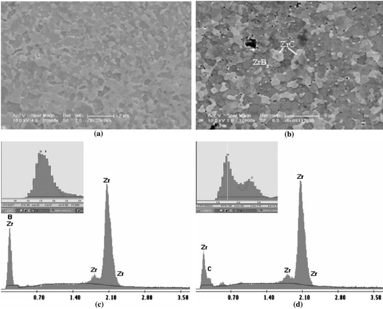
Fig. 4—SEM micrographs of the etched  $ZrB_2$ - $ZrC$  composite produced at 40 MPa, for 30 min with 1 wt pct Ni: (a) 1400 °C and (b) 1600 °C. The dark gray particles are  $ZrB_2$ , and the light ones are  $ZrC$  particles, as shown by the respective B and C signals in the X-ray spectra in (c) and (d). Spectra from two principle phases,  $ZrB_2$  and  $ZrC$ , are shown in (c) and (d) as insets at a high resolution to show the ability to distinguish the two phases based on the low-energy peaks.
