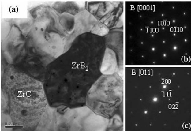
Fig. 5—(a) Bright-field TEM micrographs of  $ZrB_2$ - $ZrC$  composite produced at 40 MPa, 1400 °C, 30 min (1 wt pct Ni) with selected area electron diffraction patterns for the (b)  $ZrB_2$  and (c)  $ZrC$  phases.
