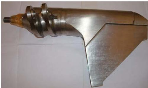
Fig-1. Titanium Torque Shaft Assembly
