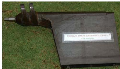
Fig-2. CFRP Torque Shaft Assembly
