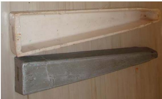
Fig-5. Aluminum core with silicon rubber cap
