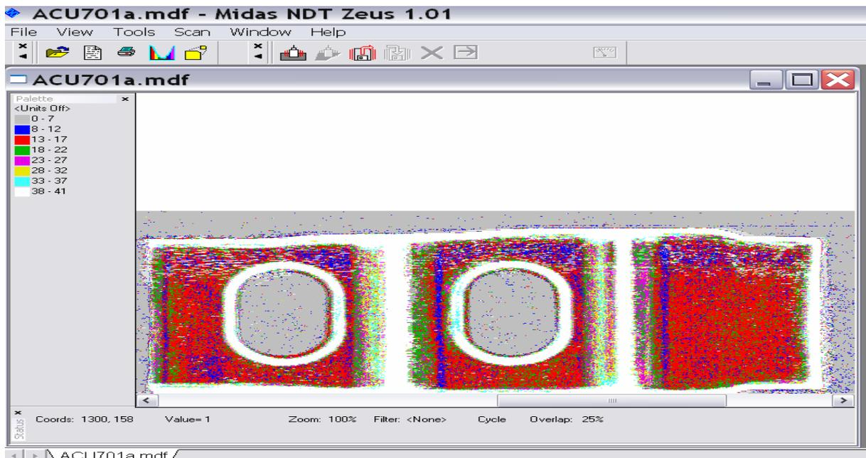
Figure-5 C-scan plot of Sub-structure
