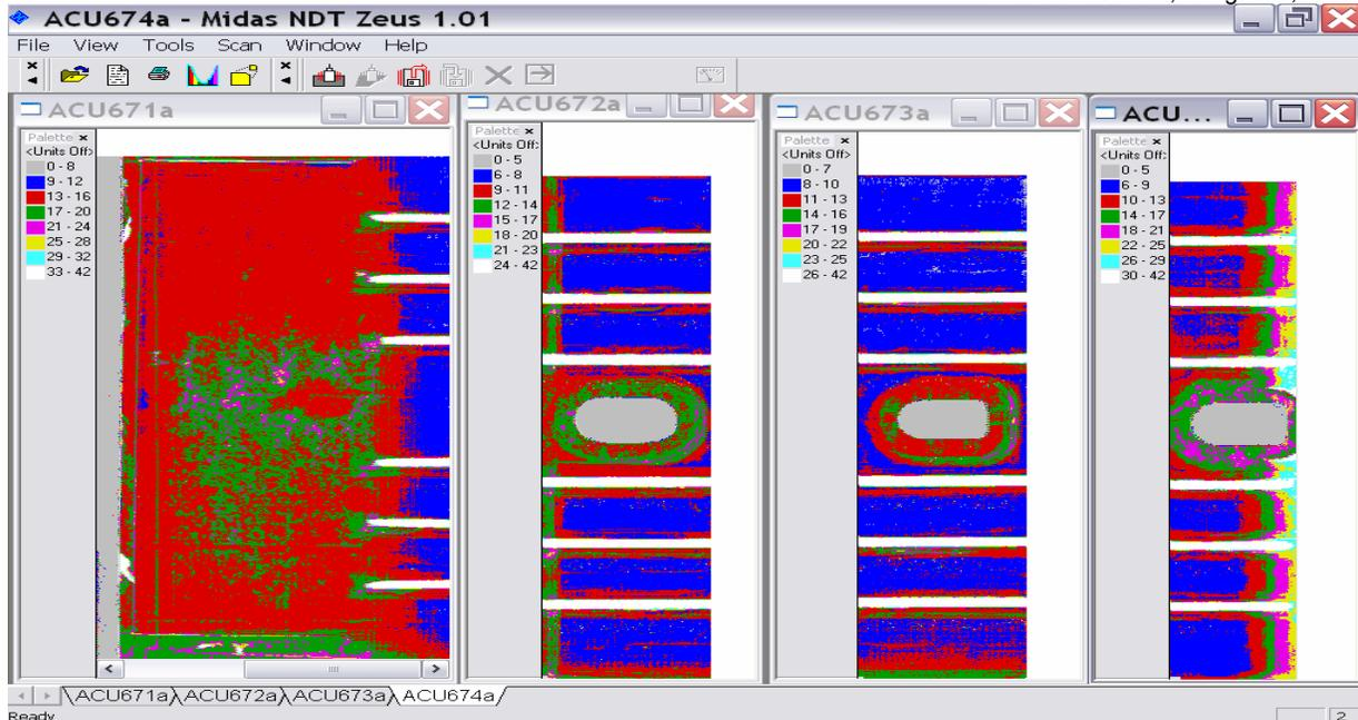
Figure-9 C-scan image of the Wing test box Bottom skin
