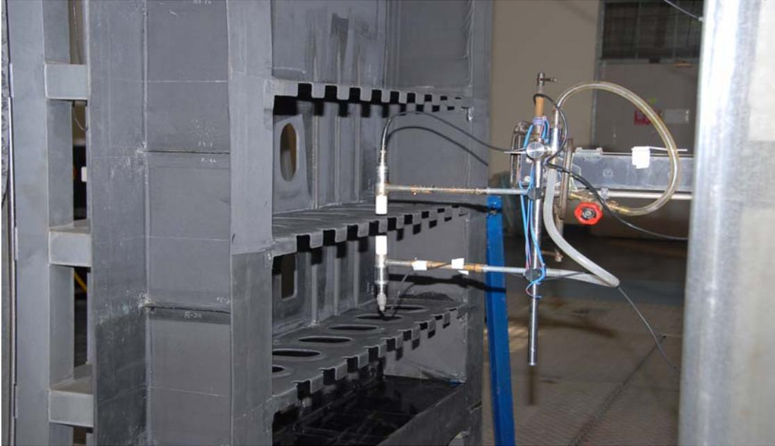
Figure-7 Test box Rib inspection
