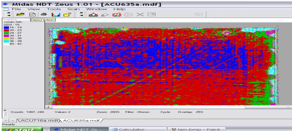
Figure-3 C-scan plot of 12mm thick Good laminate
