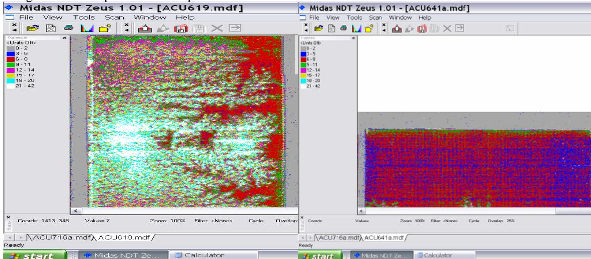
Figure-1 C-scan plot of 2.72mm thick Bad laminate
