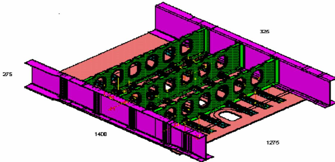
Figure-6 Co-cured wing test box
