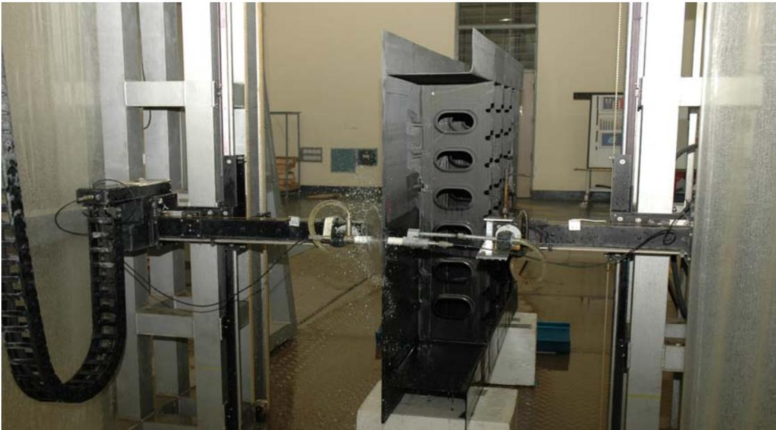
Figure -8 Test box Bottom Skin inspection
