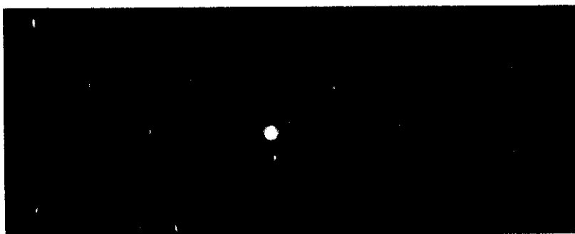
Figure 5: Oscillation photograph of the grown crystals.
