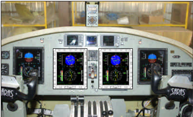
Fig. 8 Proposed MIP layout with EICAS display system for SARAS application
