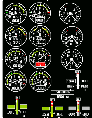
Fig. 7 Display Unit with typical symbology for EICAS
