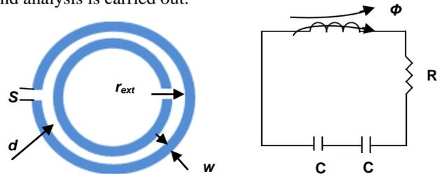
Fig. 1. Schematic of the double ring circular SSRR and its equivalent circuit
