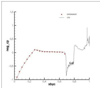
**Fig. 6.**  $C_p$  Comparison along store body at an angle of  $45^\circ$  from pylon centre line for position-43
