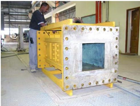
**Fig.7 Mach 3.6 water cooled nozzle**
