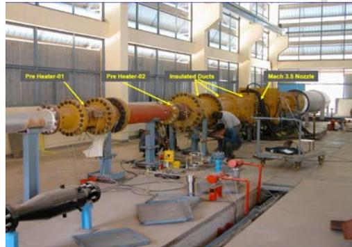
**Fig.8 Semi free-jet test rig**
