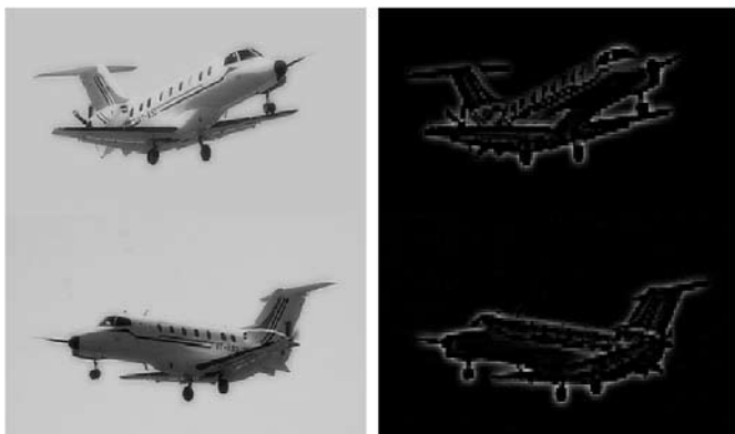
Figure 6. Fused and error image with two levels ( L=2 ) of decomposition using MSVD.
