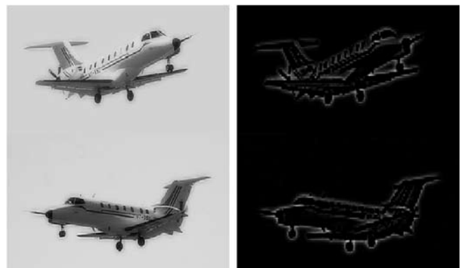
Figure 7. Fused and error image with two levels ( L=2 ) of decomposition using wavelets.
