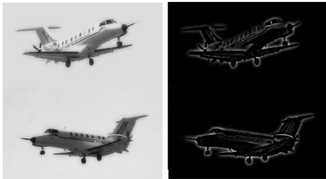
Figure 4. Fused and error image with one level ( L=1 ) of decomposition using MSVD.
