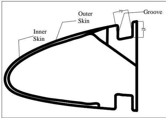
**Figure 7 Section of LE of the wing (with grooves)**
