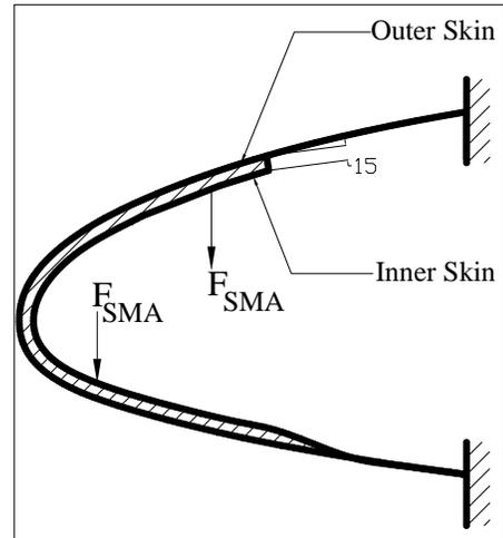
**Figure 5 Section of LE of the wing (15mm offset)**
