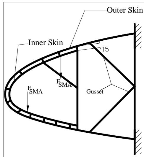
**Figure 6 Section of LE of the wing (with gussets)**
