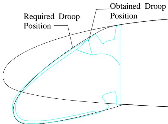
**Figure 8 Comparison of FEM analysis with required droop**
