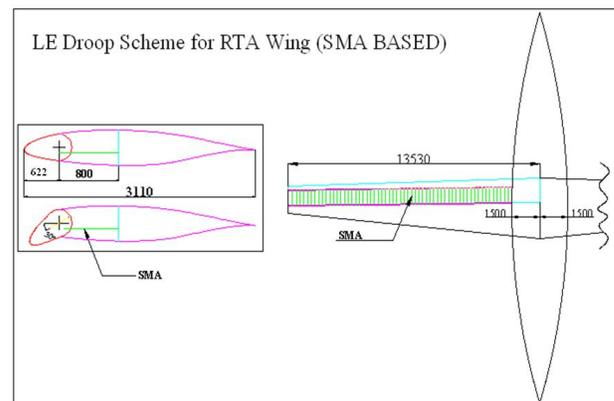
Figure 1 SMA based LE droop scheme
