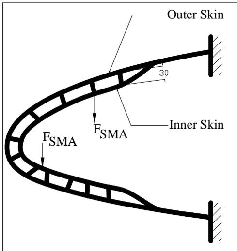
**Figure 4 Section of LE of the wing (30mm offset)**
